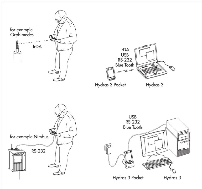
The overview shows which Hydras 3 Pocket functions are available for which dataloggers:
