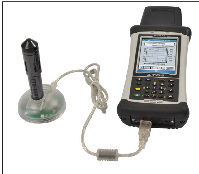
CTD-Diver datalogger shown with Diver-Pocket* software
