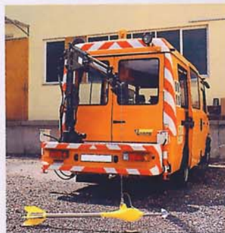
Measuring-Van with OTT- 100 kg Double drum winch and C 31 current meter.
