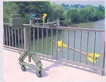
C 31 with 25 kg Single-drum winch and movable Trolley for the measurement e.g. from a bridge.
