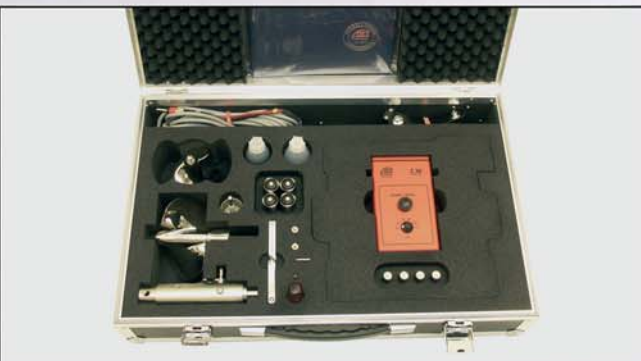
Fig. 2: Instrument case for a current meter used on rod
