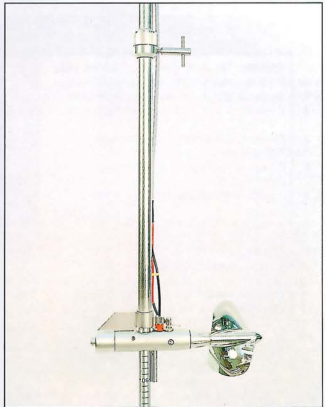
Fig. 3: C 31 current meter on rod 20 mm dia. with relocating device HERES.
