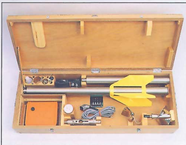
Fig. 8: Instrument case for C 31 cable-suspended meter equipment with middle piece 25 kg, 50 kg or 100 kg.
