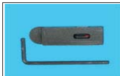
Figure 11. The Adjustable Secondary Standard includes a fluorescent rod that provides an extremely stable signal.
