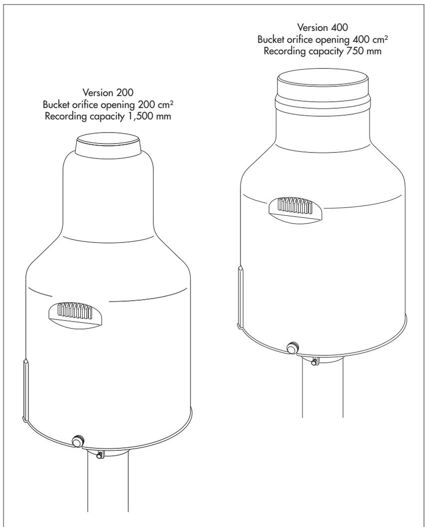
The precipitation gauge determines the weight of the collecting bucket including content every 6 seconds with a resolution of 0.01 mm (= raw data). The difference between this measurement and the base weight of the empty collecting bucket gives the current bucket content.
